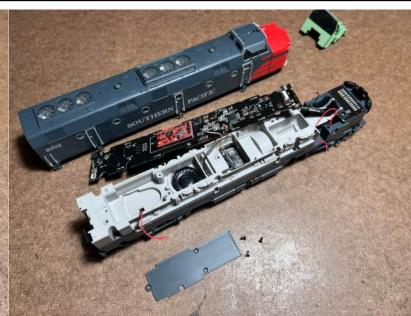
Remove the three screws and the cover of the enclosure.
