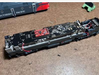
Unsolder the two rear truck wires, the two motor wires and the two speaker wires. Remove the three screws holding the PCB to the chassis.
