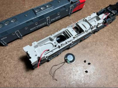
Reseat the top half ensuring the truck and motor wires are routed correctly.
