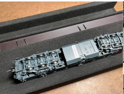
Remove the four screws holding the shell on.
