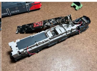
Lift the PCB. You should not need to pull the ribboncable from the PCB, but carefully handle the PCB during this process.
