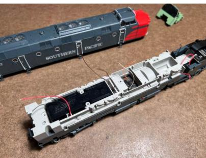
Route the speaker wires up trough the top-half passage and press the SSS speaker in place.
