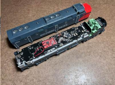
Reinstall the PCB with the three screws and re-solder all of the wires (which get re-routed through the same PCB holes). Replace the shell and attach with the four screws from step one.
